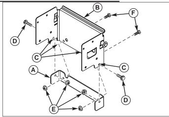
Figure 2. Frame Plate Reinforcement Installation
